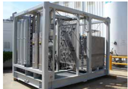
Hydraulic Power Unit
