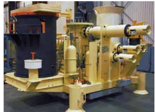
DRIL-QUIP Subsea Tree with deepwater Control Pod
