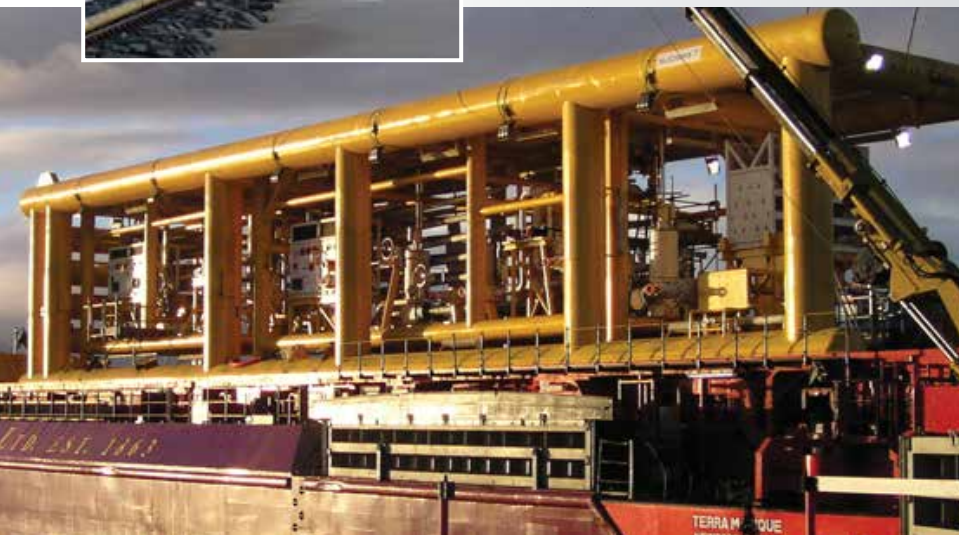
Towhead housing Subsea Production Manifold and DRIL-QUIP HIPPS destined for installation in the North Sea
